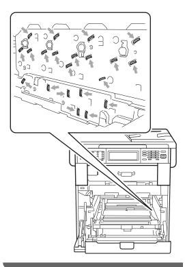
Hold the green handle of the belt unit with both hands and lift the belt unit up, then pull it out.
